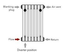
The flow must be connected on the side closest to the flow diverted.
